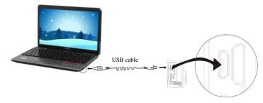
Connect the camera to the computer for charging, at this time, the charging indicator will be in blue, and it will be off after charging. Generally, it takes 2-4 hours to charge the battery.
