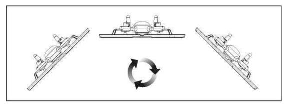
Press the flip button, and you will hear two beep tones. Move the right joystick to make the aircraft flip. When moving the joystick to the left, you will fly a left flip. Move it right to fly a right flip.
