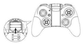
If the transmitter is not to be used for a longer period of time, remove the battery for storage.
