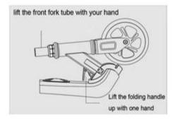
Lift the folding handle up with one hand and lift the front fork tube with the other hand and you hear a "click".
