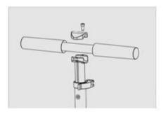
Use the screwdriver to lock the handle block.
