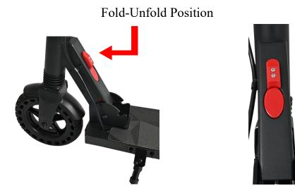
Push up and press the red button to fold or unfold the Electric scooter.
