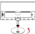
4. Place the monitor on a level and stable platform after the assembly has been completed.
